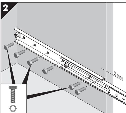
Affix nuts & bolts to the slides inside of the cabinet unit through slide holes and make sure both slides are mounted vertically and horizontally parallel. Use as many nuts & bolts as you think is necessary for the cabinet unit.
