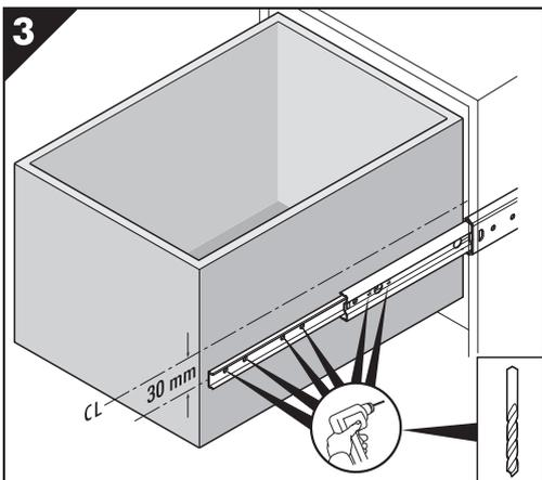
Marking holes to fix the internal member of the slide to the drawer. When marking hole placements you **MUST NOT** drill through the slide holes during installation. Doing this will create metal filings which lodge in the tracks resulting in rough running and ultimately, failure of the slides.
